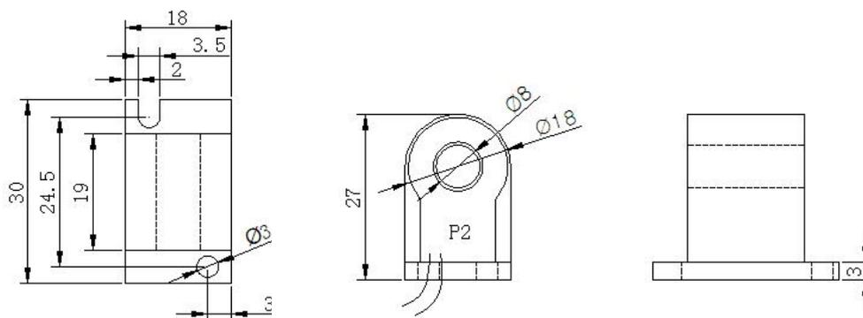
Note: The primary current enters from P1 and exits from P2 (glue filling surface). The red and yellow lead lines are S1 and S2. The length of the lead line is  $2\text{m} \pm 10\text{cm}$ .
